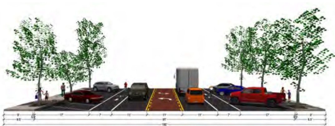
Rendered Section of Rightsizing Configuration
